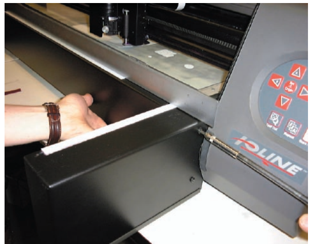
Fig. 2 - Place a ruler on the white strips while tightening the mounting screws.
