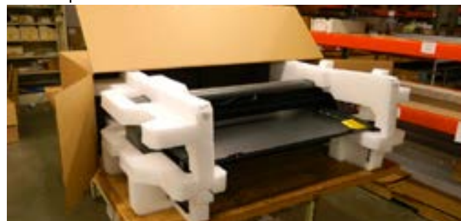
Step 14: All 4 foam pieces are correctly and securely installed. The 300/350 is shown partially pushed into the carton.
