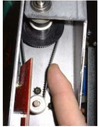
Transmission belt (The correct tension)
