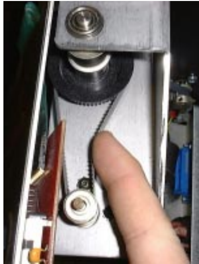
Transmission belt (Very loose)
