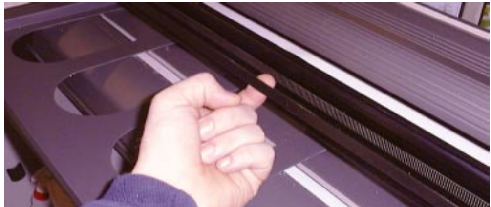
“Y” axis drive belt Pull to see if it's tight (Move the knife carriage to the right side of the machine).
