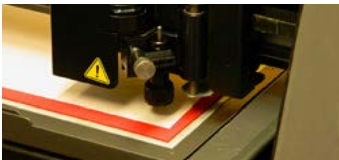
Step 7: Lay out the fabric on the 300/350 tray with the backing material side up as shown. NOTE: The tack material that is used to hold the fabric to the 300/350 tray depends on the fabric used.
