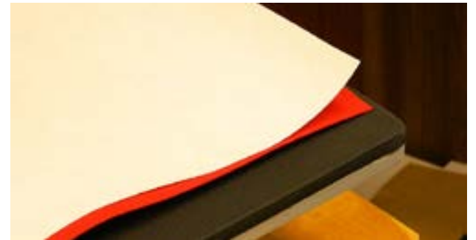
Step 4: This shows how the double sided backing is adhered to the fabric. It is pressed onto the fabric by the heat press.
