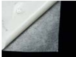
Step 3: A close up of the Double sided backing (left photo) compared to the Single sided backing (right photo). The double backing is thinner in feel and has a linear/fibrous look to the surface.
