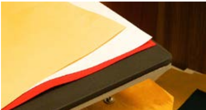
Step 5: This shows the 3 layers that is needed before pressing with heat and pressure. The fabric (red), the backing (white) and the (yellow) the protection layer.
