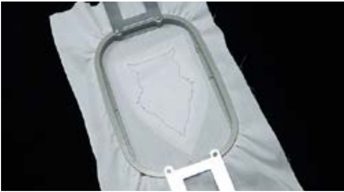
Step 11: Create a placement stitch on the fabric in the hoop. Then place the fabric within the outline placement stitch as shown.
