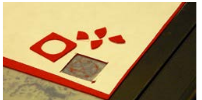
Step 8: Create a test cut first to determine the proper blade depth, force and cut quality.
