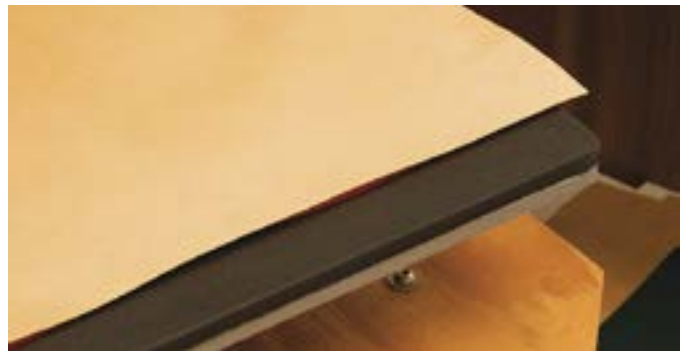
Step 6: Heat press 300 degrees for 10 seconds, while using medium pressure. You can now open the press and remove the craft paper and the fabric.
