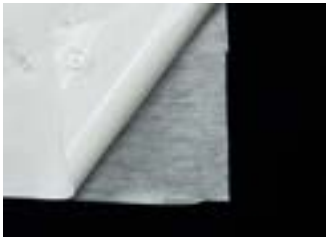
Step 3: A close up of the Double sided backing (left photo) compared to the Single sided backing (right photo). The double backing is thinner in feel and has a linear/fibrous look to the surface.
