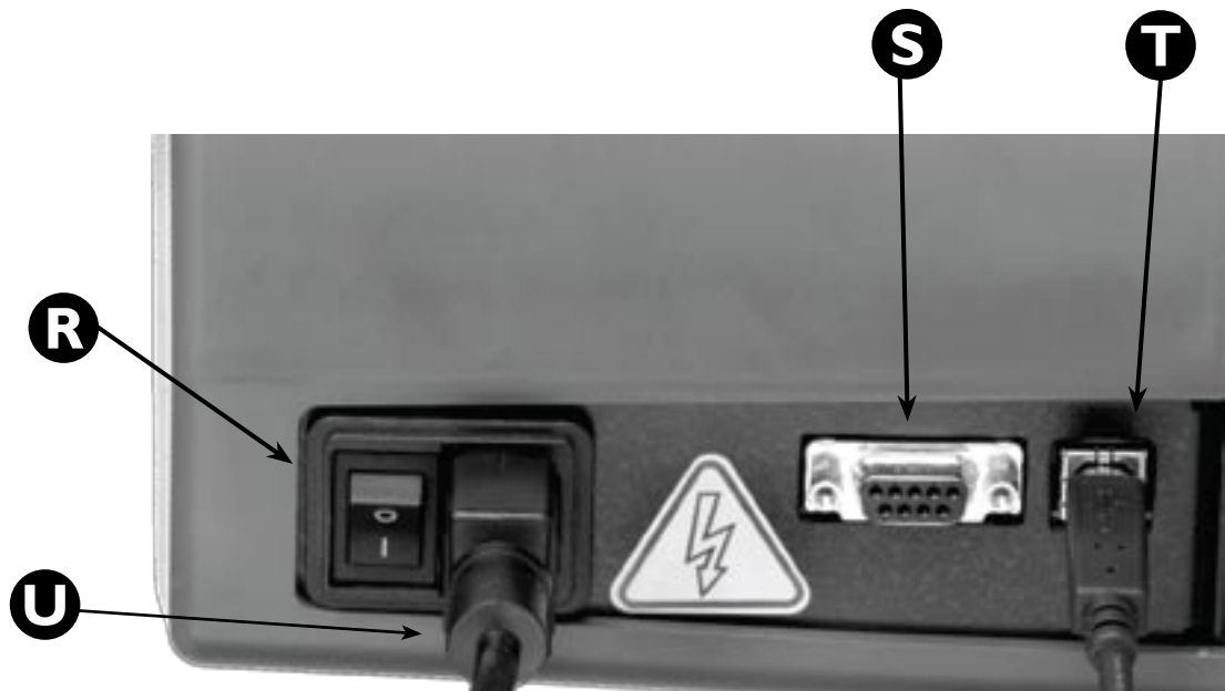
Figure 2. Power and communications ports on the Ioline SmarTrac SC-72 are located on the back of the right cover.
