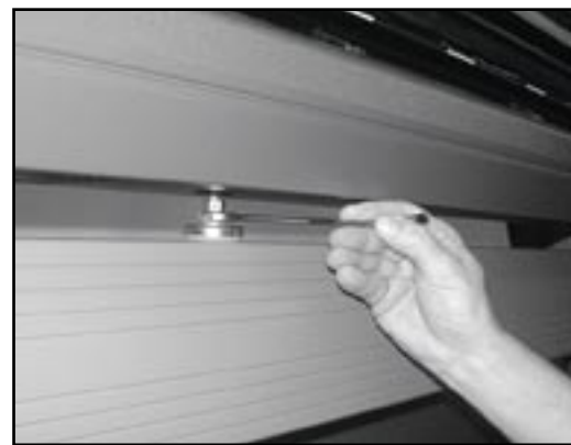
Figure 16. Adjust the platen height with the leveling pads using a \frac{1}{2} -in open-ended hex wrench. Careful adjustment helps maintain proper media alignment.
