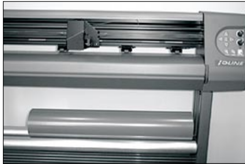
Figure 15. Material loaded on media roller.
