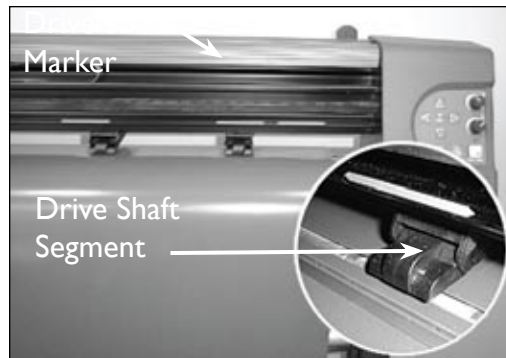
Figure 16. Place pinchwheels under drive shaft markers.
