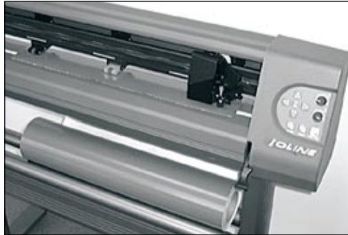
Figure 18. Leave slack in the material.
