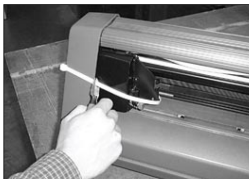
Figure 11. Remove packing foam and plastic strip.
