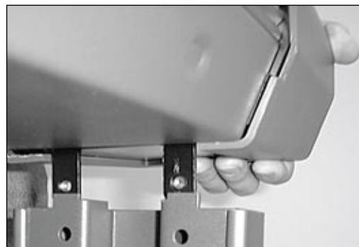
Figure 8. Place cutter on stand.
