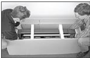
Figure 4. Proper lifting procedure. Requires two people.
